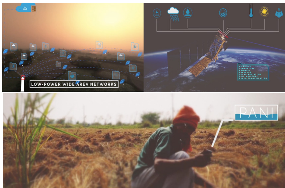
Figure 1. Schematic showing the main components of PANI based on satellites and weather models (upper right) combined with low-cost ground sensors in a LPWAN network (upper left) that produce plot scale irrigation advisory for the farmer (lower panel).
