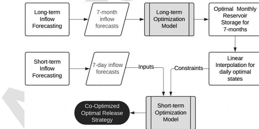
FIG. 6. Schematic explaining the procedure of co-optimization with the long- and short-term objectives.
