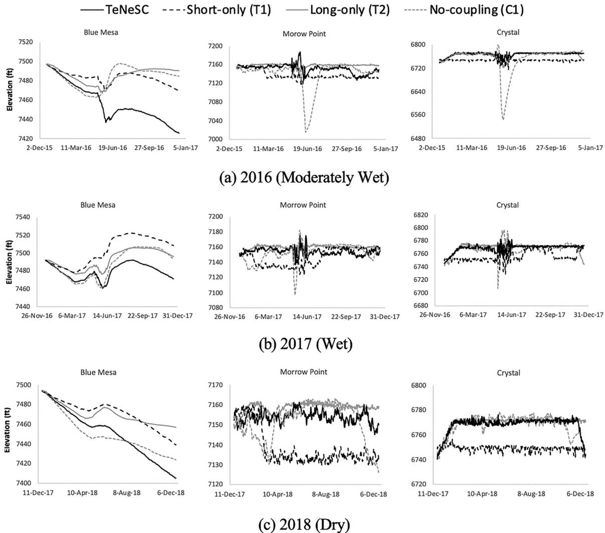
FIG. 7. Optimal reservoir elevations from the different strategies using the perfect forecast scenario for the three dams over the three years with different flow characteristics.
