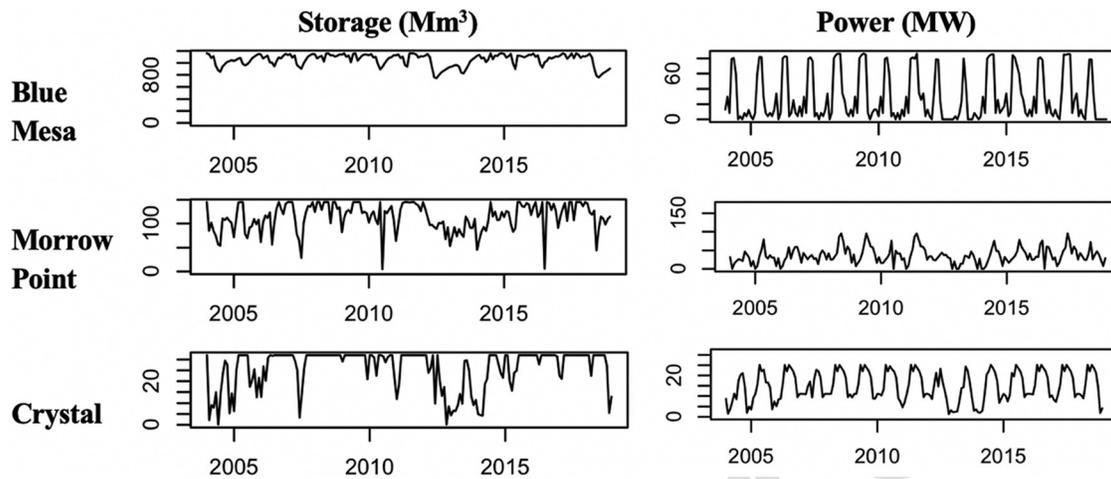
FIG. 9. Benchmark control rules designed specifically for hydropower maximization using the R package *reservoir* for the dams in the Aspinall Unit during the period 2004–2018 at the monthly scale (after Turner and Galelli, 2016).
