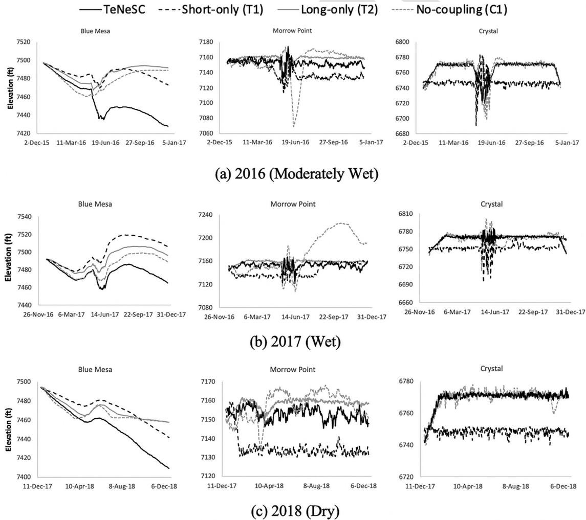
FIG. 8. Optimal reservoir elevations from different strategies using operational forecasts (ANN/linear regression-based) for the three dams.
