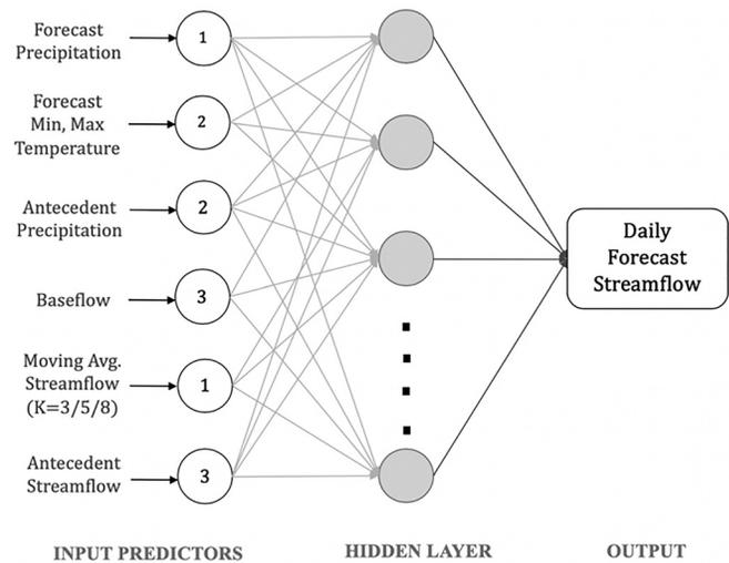
FIG. 4. ANN model configuration with the selected input predictors for daily streamflow forecasting over the Blue Mesa dam. Log sigmoid and linear transfer functions were used for hidden and output layers, respectively. The number of antecedent/forecast days for each node is also shown. K is the window length for moving average streamflow that varies with the forecast lead time.
