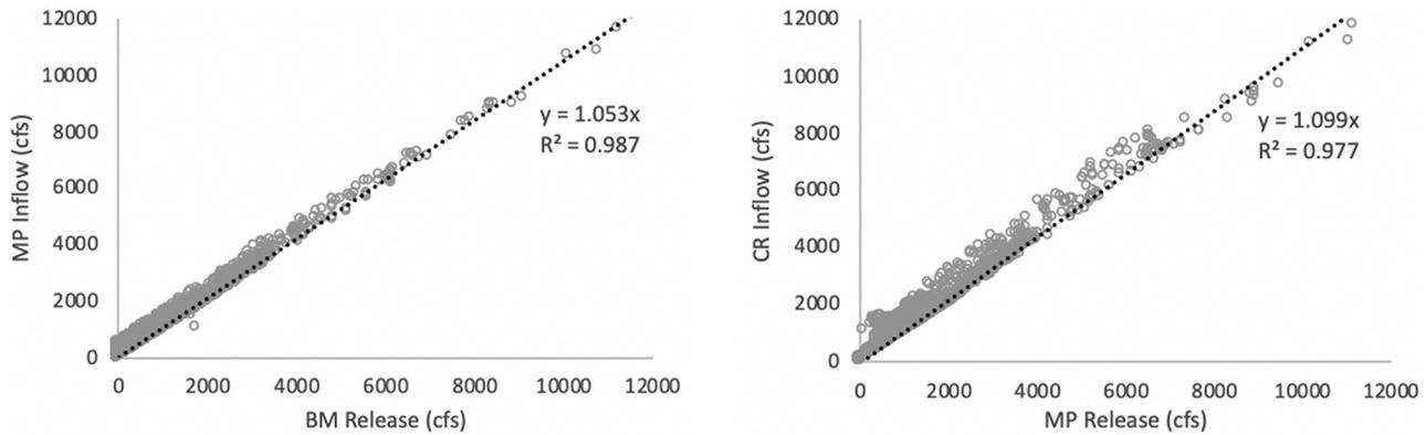
FIG. 5. Scatter plots showing linear regression between release and inflow of the upstream–downstream dam pairs of Blue Mesa (BM)–Morrow Point (MP) and Morrow Point (MP)–Crystal (CR) dams.
