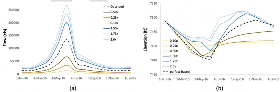
**FIG. 10.** (a) Perturbed inflow timeseries for the Blue Mesa dam over 2016 to be used for the TeNeSC scheme; (b) optimal monthly elevations for the Blue Mesa dam using the long-term optimization model based on the different perturbed forecast inflow time series; the black dashed line is based on perfect forecasts (i.e., observed inflow).
