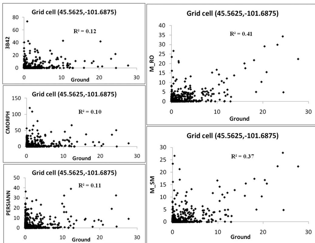
FIG. 9. Scatterplots of ground observation vs satellite rainfall data at a particular grid cell. It shows the improvement of correlation coefficients of the merged satellite products for the period of 2004–05.
