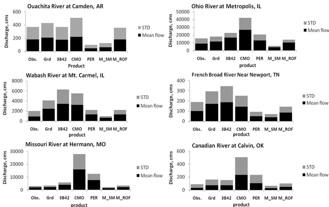
FIG. 6. Statistical comparison (mean and standard deviation) of observed and simulated streamflow from various rainfall products for the period of 2004–05. The area of each subbasin is shown in Table 1. The following are were shown (abbreviated accordingly): standard deviation, observed streamflow, gridded GV rainfall, 3B42-RT satellite product, CMORPH, PERSIANN-CCS, M\_SM, and M\_ROF.
