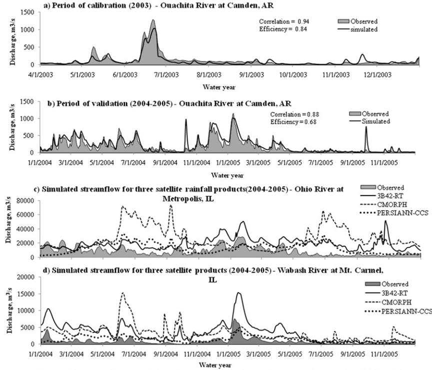
FIG. 3. Streamflow simulation performance of various rainfall products. (a) Calibration and (b) validation sample results for the VIC model using GV rainfall data on the Ouachita River at Camden, Arkansas. (c),(d) Simulated streamflow from three satellite rainfall products (3B42-RT, CMORPH, and PERSIANN-CCS) on the Ohio and Wabash Rivers, Illinois.
