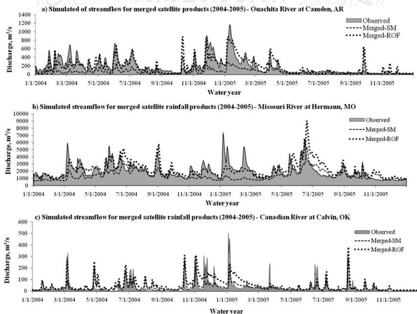
FIG. 5. Comparison of observed and simulated streamflow from two merged satellite products at three streamflow gauging stations.
