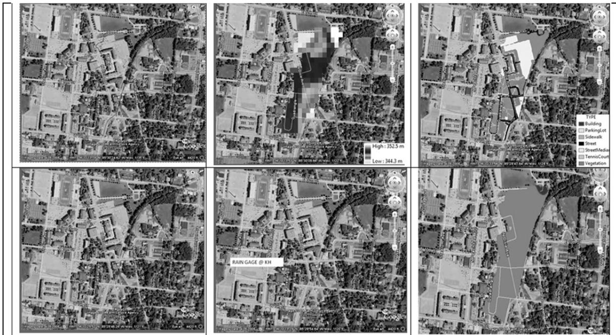
Figure 5. The six GIS layers on TTU BP watershed rendered as Google Earth KML files for display in HydroViz-TTU adaptation. Each layer in a panel represents a hydrology topic. From upper left (clockwise): General watershed boundary, elevation/terrain, land use/land cover; watershed outlet, instrumentation and soil coverage.
