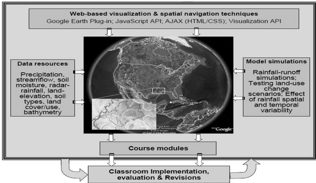
Figure 2. Overall architecture of HydroViz developed by Habib et al.[5] depicting the various inputs and modules. (figure reprinted with kind permission from Habib et al. (2011))
