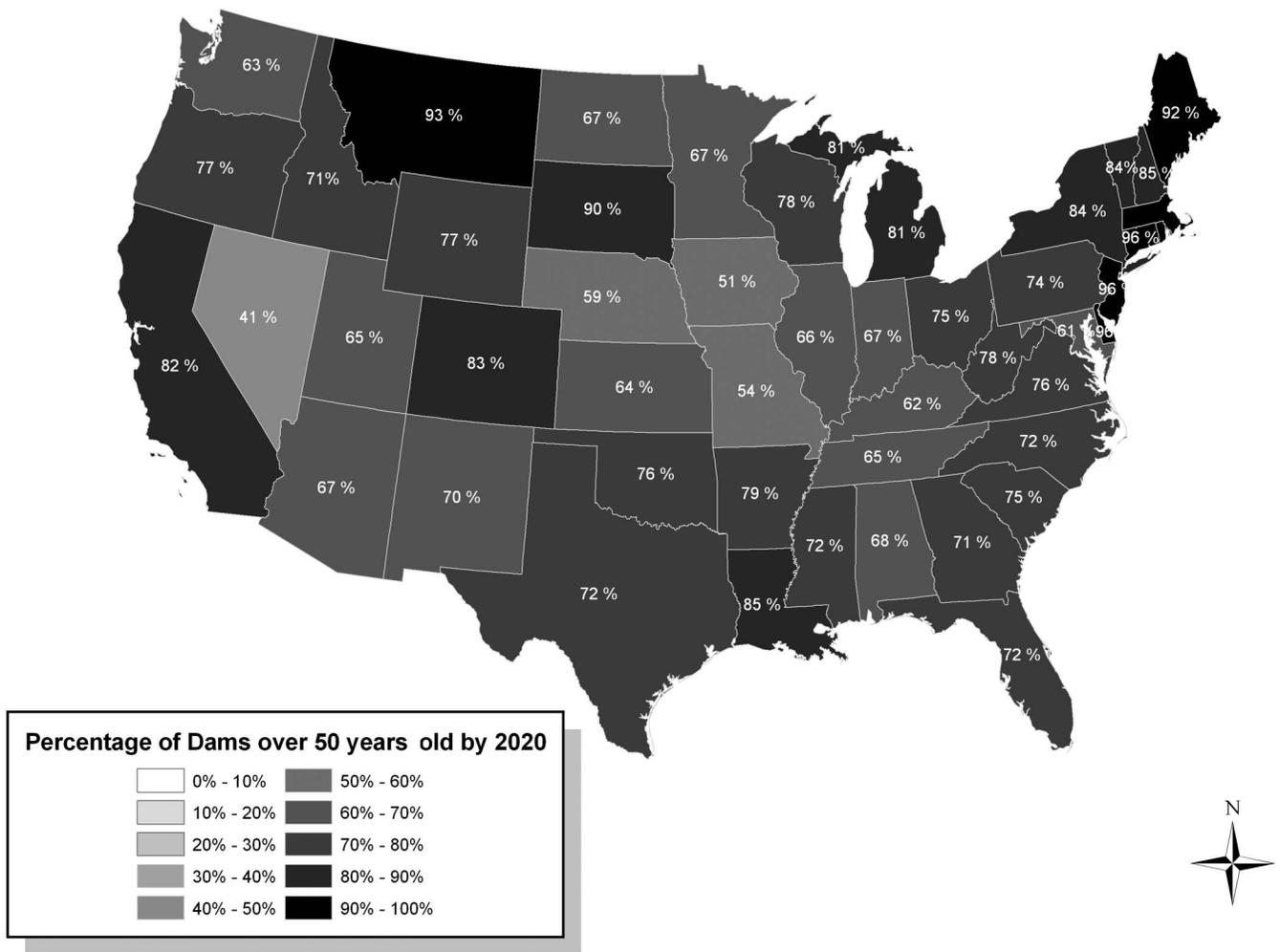
**Fig. 2.** Percentage of dams per state that will be over 50 years old in 2020 [Reprinted from Hossain et al. (2009); data source: National Inventory of Dams of USACE]
