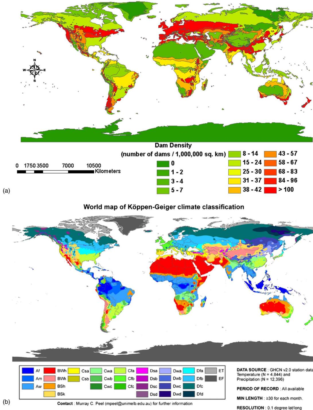
**Fig. 8.** (a) Dam density (number of dams per 1 million square kilometers) for each major Köppen climate zone (climate class not shown) on the basis of the GRanD database of 6682 dams; and (b) the major Köppen climate classes reproduced from Peel et al. (2007) with kind permission provided
