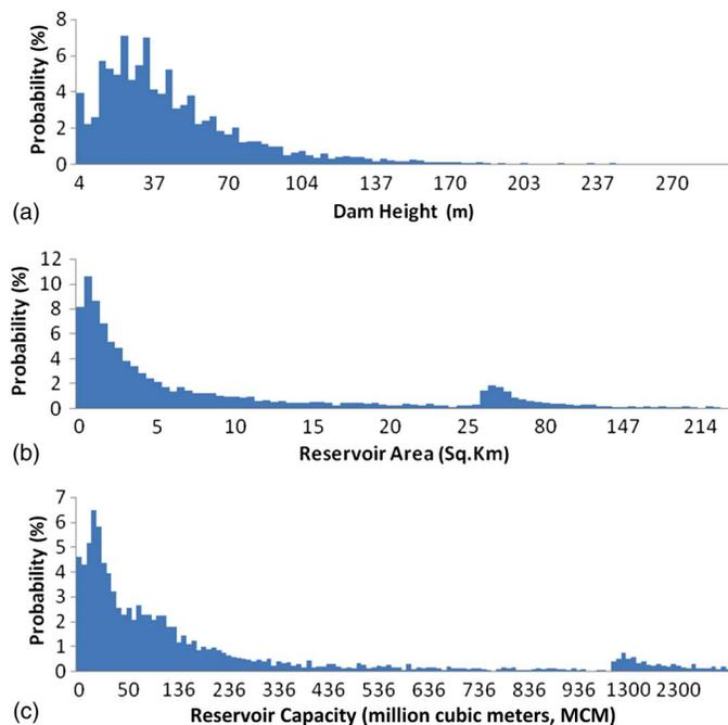
**Fig. 12.** Probability distributions on the basis of the GrandD database; (a) dam spillway crest height; (b) surface area; and (c) reservoir volume
