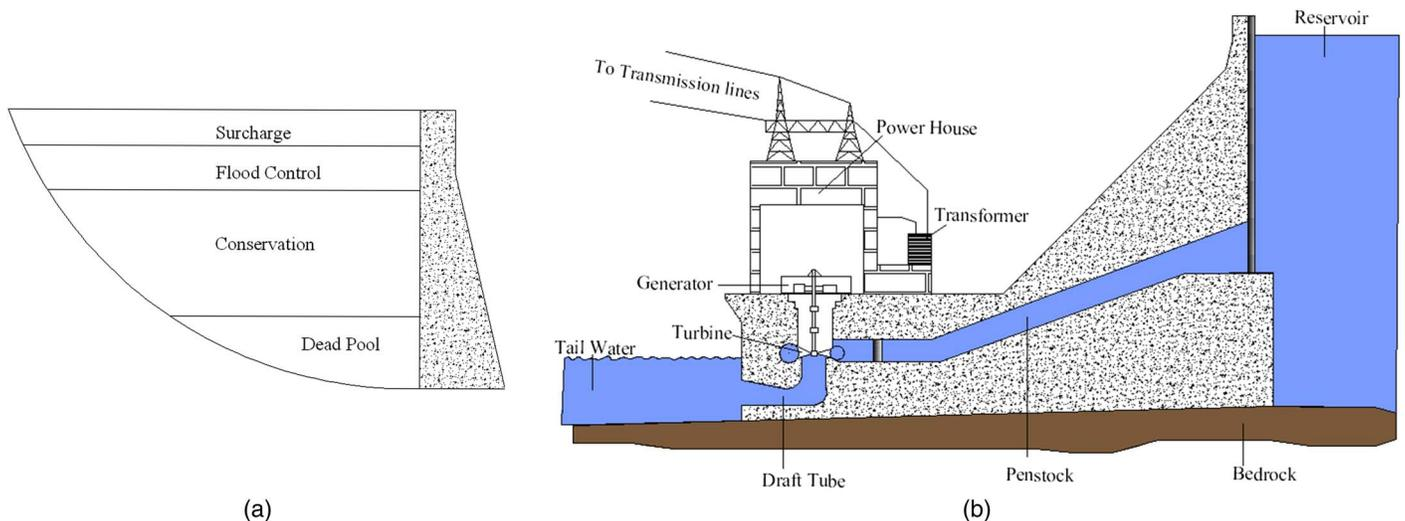
**Fig. 7.** (a) Typical pools allocated during dam design, planning, and operations; (b) hydropower generation plant showing how power generation can be reduced by a lowering of the reservoir level to make way for other pools
