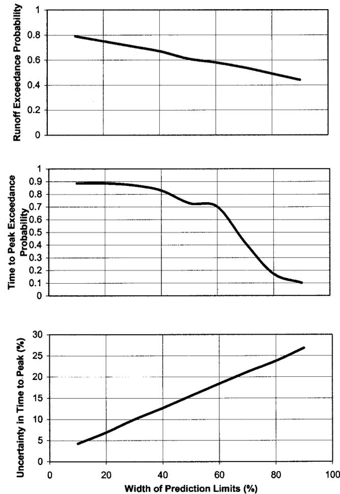
**Fig. 6.** Runoff and time-to-peak exceedance probability (upper and middle panels) versus width of prediction limit (upper-lower quantile range); lower panel: uncertainty in time-to-peak versus width of prediction limit
