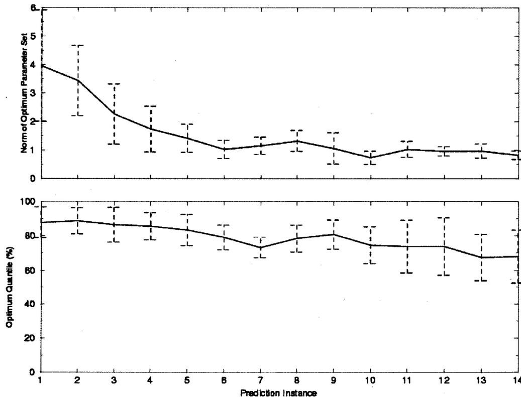
**Fig. 7.** Mean and one standard deviation (vertical bars) of the norm of optimum parameter set (upper panel) and optimum quantile (lower panel) versus prediction instance
