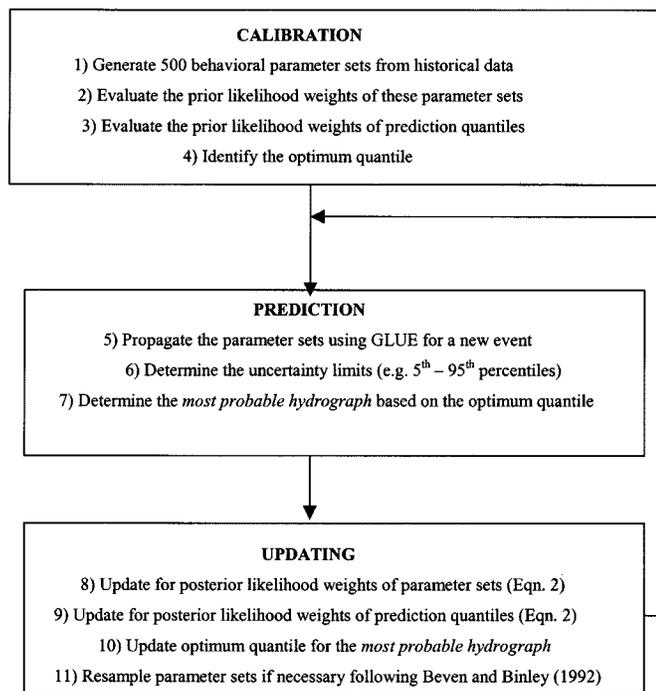
Fig. 3. Flowchart for the probabilistic discharge prediction scheme
