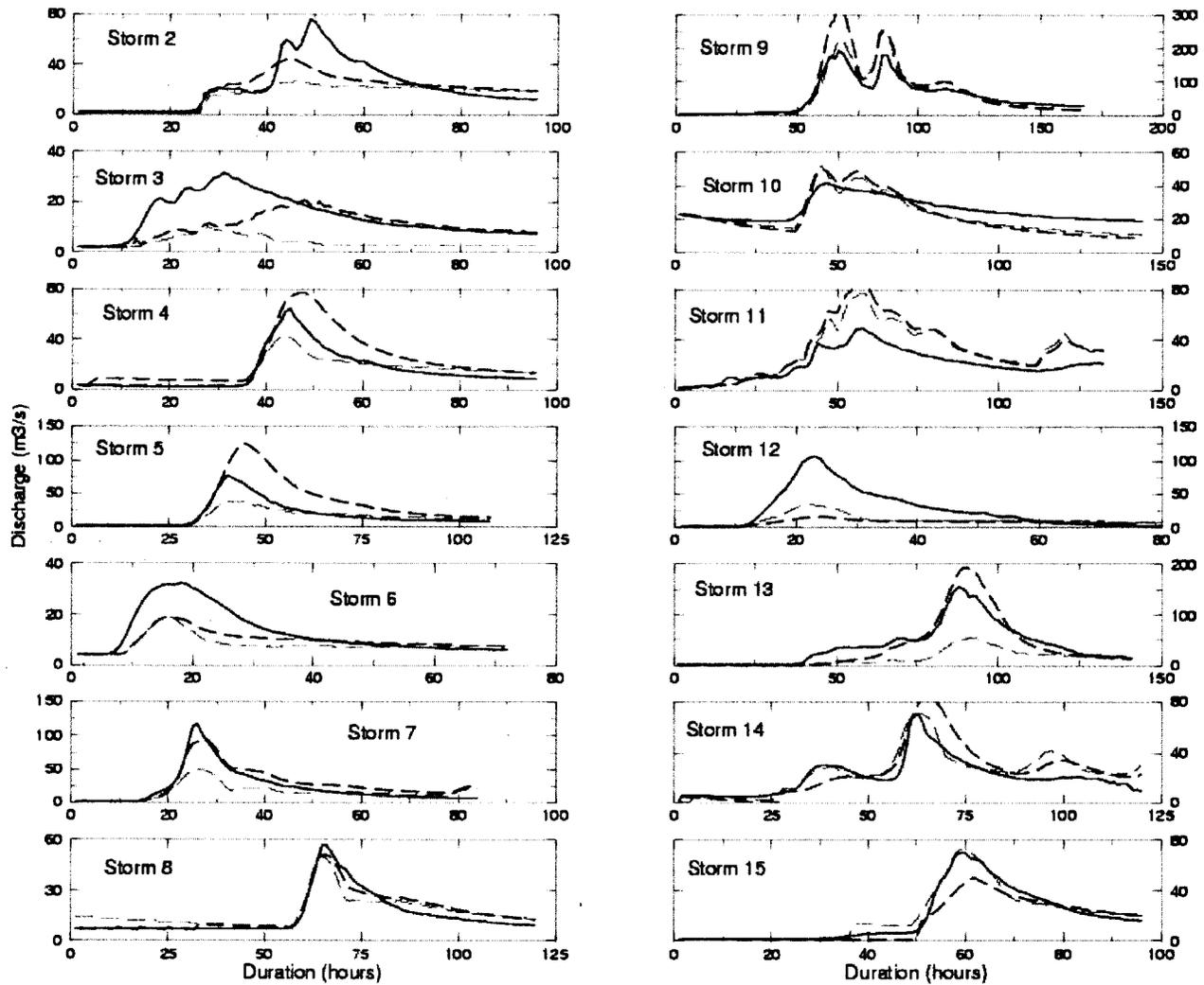
Fig. 4. Observed (solid line) versus predicted runoff hydrographs derived from deterministic (thin dashed line) and probabilistic (thick dashed) schemes for chronological sequence of 15 storm events
