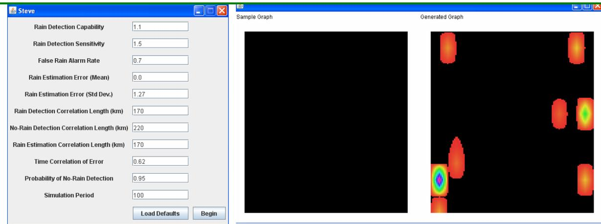
**Figure 1.** The STEVE (Ver 1.0) GUI currently developed at TTU for teaching stochastic theory in the classroom for water resources engineering. Left panel is the control panel where user keys input parameters for various stochastic theory concepts. Middle and right panels visualize on the basis of user-driven input. A control visualization (middle panel) for ‘default’ parameters is also created to visually observe the effect of altering a stochastic parameter.
