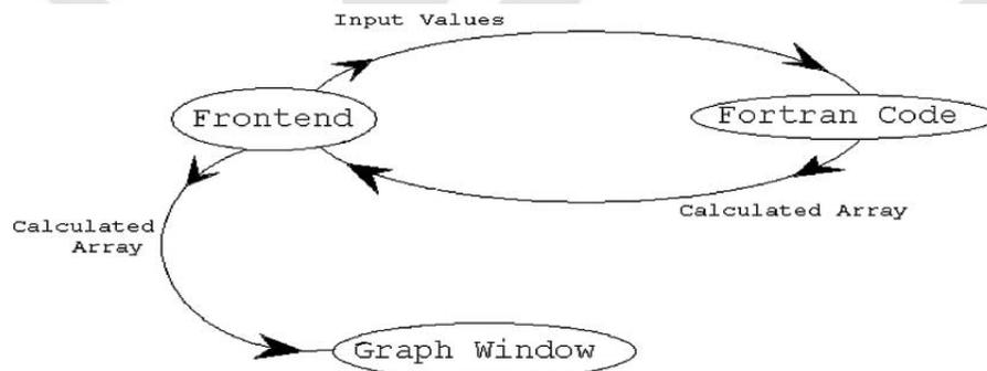
**Figure 2** Entity dependency diagram for prototyping the *SREM2D*-GUI. Front end is programmed using Java Native Interfacing (JNI) language.
