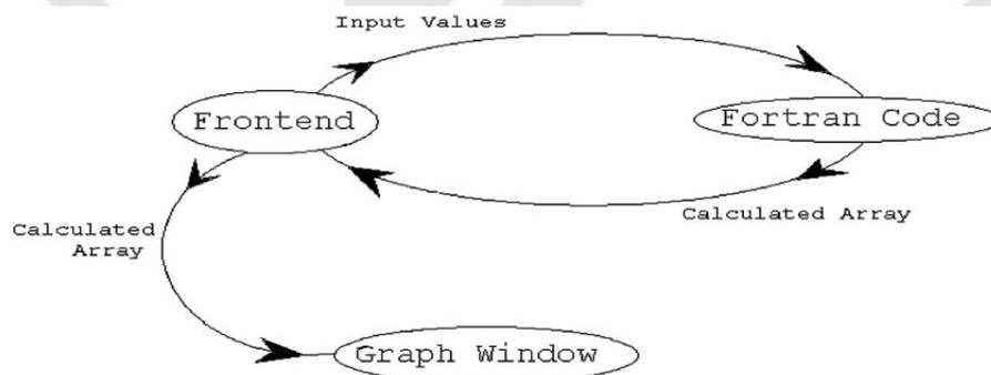
**Figure 2** Entity dependency diagram for prototyping the *SREM2D*-GUI. Front end is programmed using Java Native Interfacing (JNI) language.
