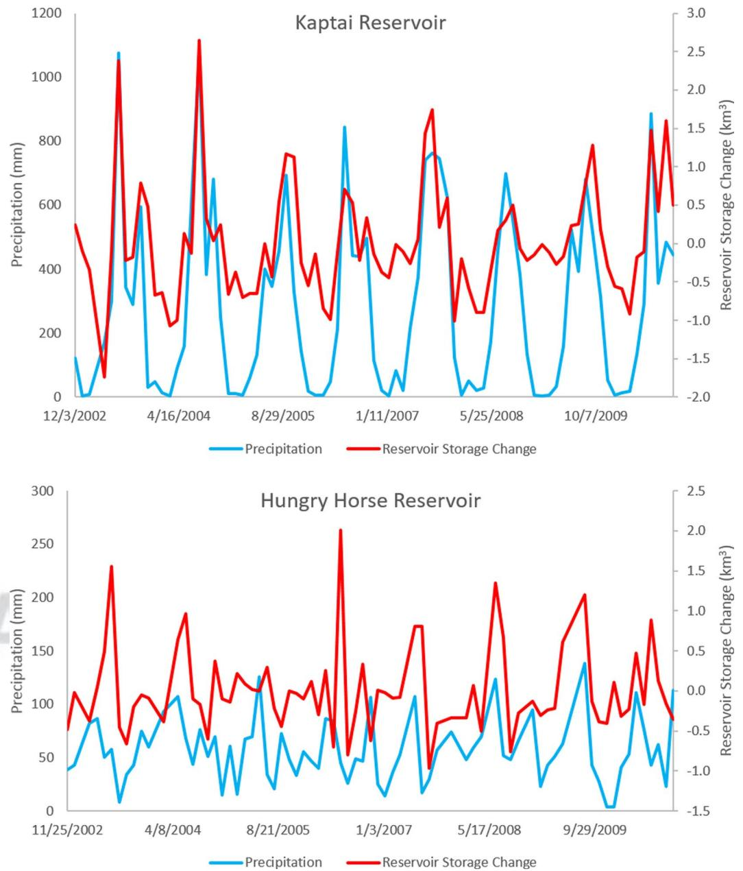
**Figure 4.** Precipitation and reservoir storage change for (top) Kaptai Reservoir and (bottom) Hungry Horse Reservoir. Precipitation is summed over the 35 day period between satellite overpasses. Storage change is the difference between the total amounts of water in the reservoir between two consecutive satellite overpasses, every 35 days.
