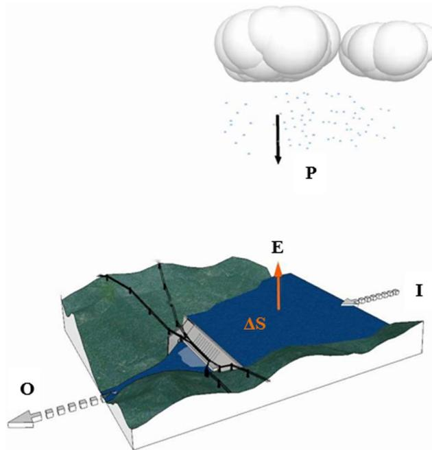
**Figure 1.** Schematic of mass balance between reservoir outflow (O), evaporation (E), changes in reservoir storage ( $\Delta S$ ), and runoff-derived inflow (I) driven by precipitation (P).
