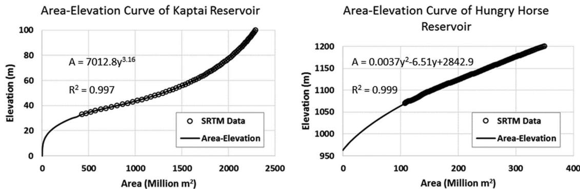
**Figure 3.** Area-Elevation curves for (left) the Kaptai Reservoir and the (right) Hungry Horse Reservoir. Note that the datums of both elevation measurements are the same and that Hungry Horse Reservoir is approximately 1000 m higher in elevation than Kaptai Reservoir.
