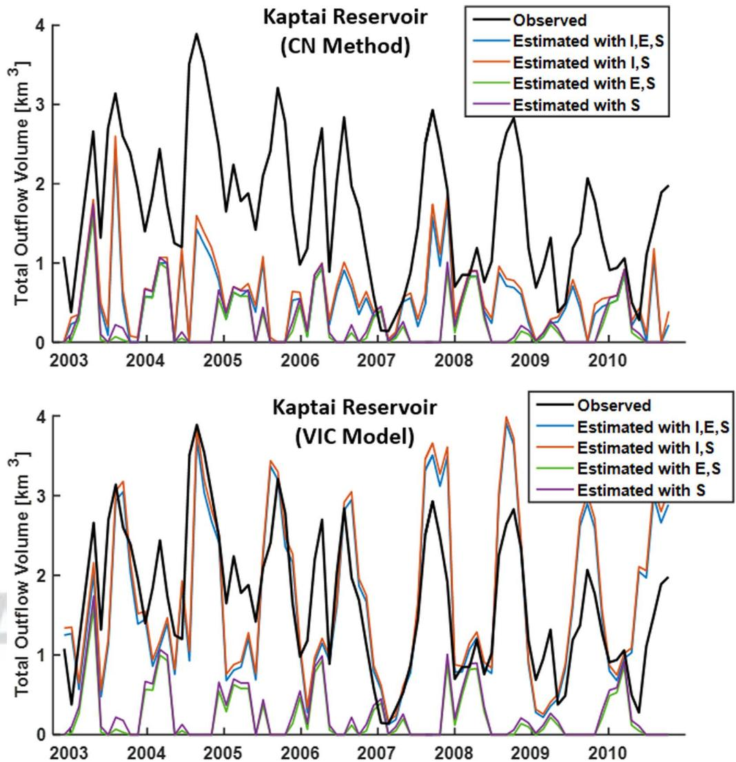
Figure 5. Hydrographs comparing Kaptai Reservoir discharge observations to discharge estimates using different components of the mass balance, changes in storage (S), runoff inflow (I), and evaporation (E). The inflow in the top graph uses the CN method while the inflow in the bottom graph uses the VIC model.
