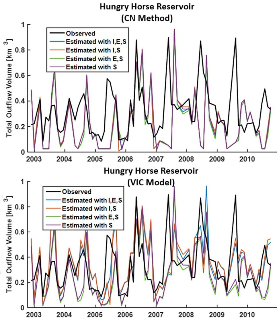
**Figure 6.** Hydrographs comparing Hungry Horse Reservoir discharge observations to discharge estimates using different components of the mass balance, changes in storage (S), runoff inflow (I), and evaporation (E). The inflow in the top graph uses the CN method while the inflow in the bottom graph uses the VIC model.
